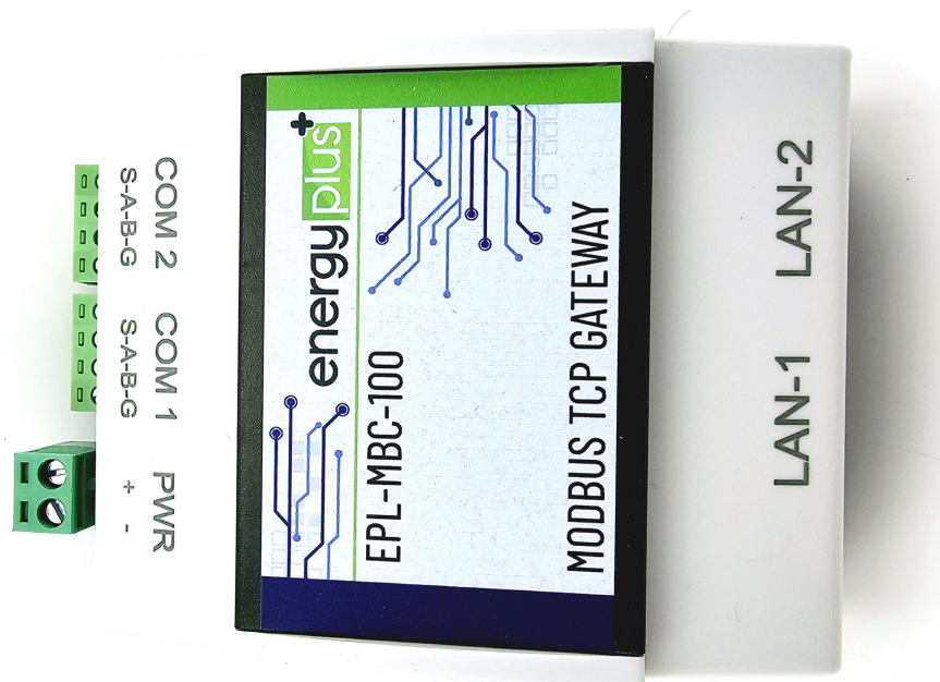
Figure 1.1 – EPL-MBC-100 front panel view
